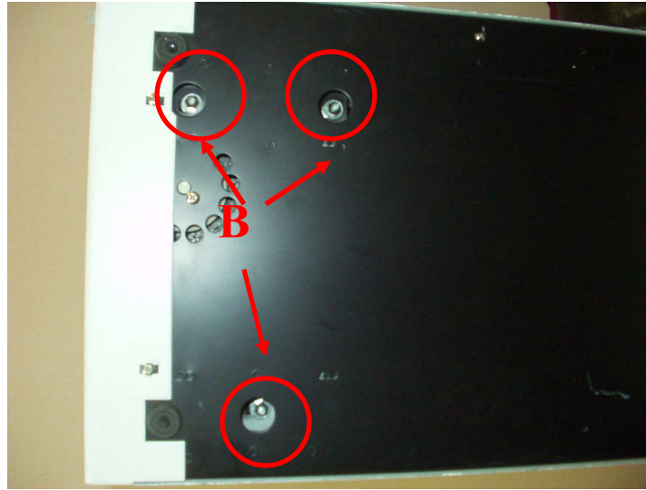
Figure 2: Mounting Screw Location on the Optics
