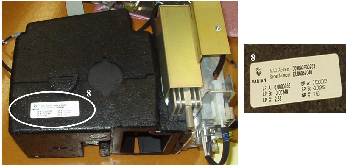
Figure 6: Calibration Coefficients on the Optics
